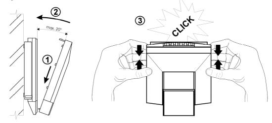
Figure1: Device mounting
