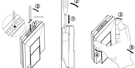
Figure2: Device demounting
