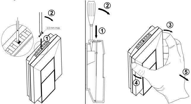
Figure 2: Device demounting
