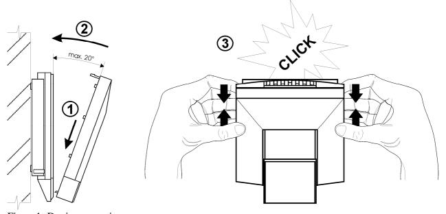
Figure 1: Device mounting
