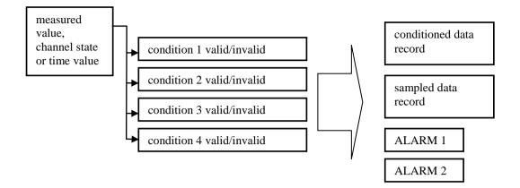
Data logger enables to set condition depending on measured value, on time and condition, which validity is remotely controlled. Each from four conditions it is possible to switch on for evaluation. Binary inputs has lower number of possibilities to set conditions, setting is analogical.
