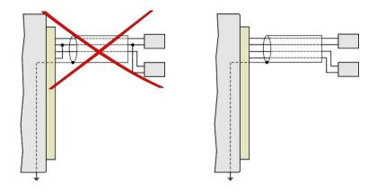
• It is recommended to earth data logger at one point – there is a special terminal on power terminal. This earthing will work correctly, if system would not be grounded at other point at the same time.
