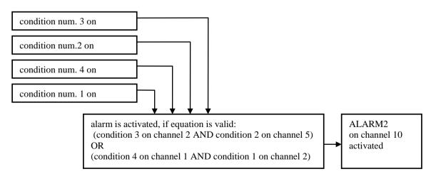
Alarm is active, if input conditions are valid. By means of combination of conditions you can solve also complex situations including remote control. Some actions last during all alarm time (audible indication, ALARM OUT output activity, visual indication, relay closing), other actions last only at the moment of alarm creation (SMS message, e-mails). Changes of ALARM OUT output state or all alarms state can be recorded.
