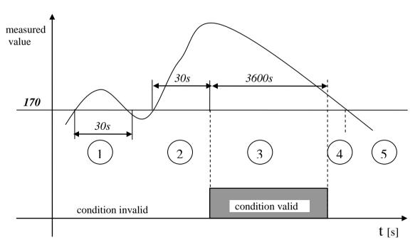
To renew validity of condition measured value first must drop below specified limit and then to exceed the limit.
