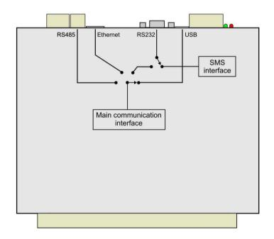
Communication interface can be selected from data logger keyboard or by means of PC program.
