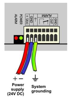
If system is not grounded properly, it is a danger of state, when system floats on variable potential against all other circuitry. It can cause communication dropouts, occasional resets and in extreme case damage of some peripherals. Especially when using pulse power sources (e.g. A1940) it is strongly recommended to ground the system.
