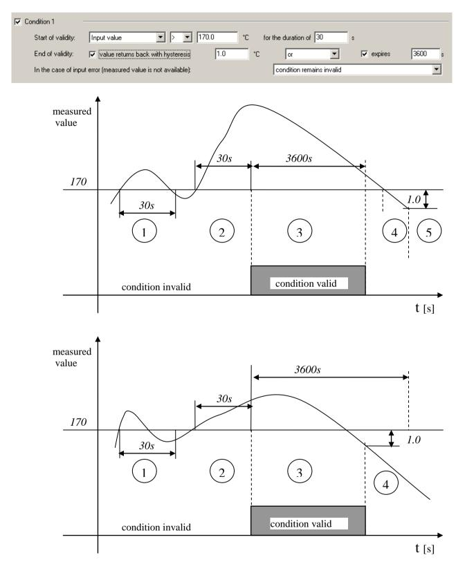
To renew validity of condition measured value first must drop below specified limit and then to exceed the limit.
