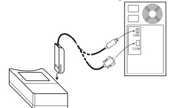
After connecting the logger to the computer reading of logger info is enabled by means of the PC software and also setting of the instrument accordingly to the user needs (menu *Configuration / Setting of instrument parameters*). Before logging start it is necessary:
