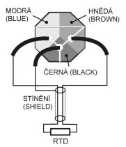
It is possible to order as an optional accessory connector for connection of temperature probe. Probe cable should be shielded, round cross section of minimum diameter of 3.5 mm and maximum diameter of 5 mm, maximum length of 10 m and as large as possible cross section of cords (stranded wires). Outer diameter must be from 1 to 1.55 mm including insulation. Connect connector to temperature probe accordingly to the figure by means of the manual included in delivery.
