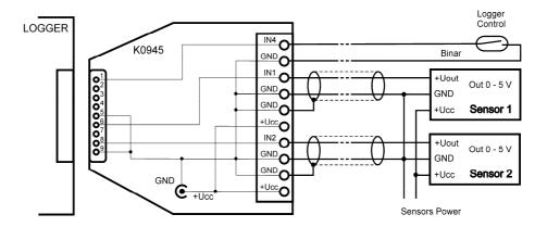
Connection to sensor signal. Power supply is located near the logger:
