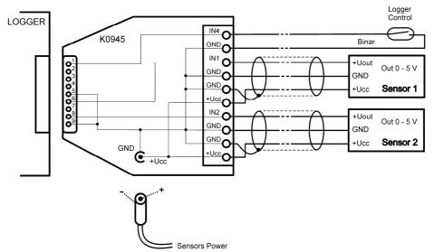
At this case sensor is possible to power e.g. from ac/dc adapter, connected via coaxial power connector to K0945 adapter. Supply voltage and the power of the applied ac/dc adapter depend on types of connected sensors.
