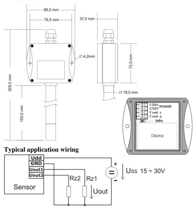
Maximum load current of each voltage output is 0.5 mA
