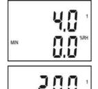
Range and type of value for output 1 (current loop I1 = symbol ,,1"on display). Type of value, assigned to output 1, is indicated by displayed unit (here %RH = relative humidity). Upper line displays current value corresponding to measured value (lower line).
