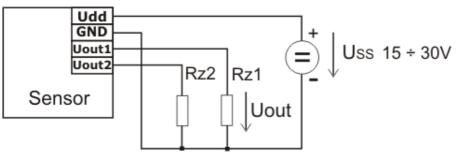
Maximum load current of each voltage output is 0.5 mA
