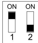
Figure 11 Switch no. 1 position for default setting restore procedure
