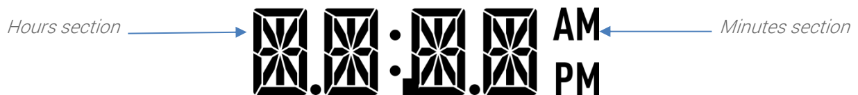
Figure 12 14-segment displays the block for time displaying
