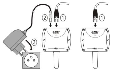
Web Sensor P8631 connection (power supply adapter, Power over Ethernet):
