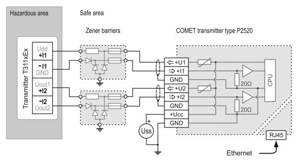
Example of the T311xEx transmitter connection to the inputs of monitoring and data logging system MS55 (COMET) using Zener barriers type JBB 7087+ (MM GROUP)
