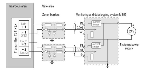
Example of the T311xEx transmitter connection to the inputs of monitoring and data logging system MS6 (COMET) using Zener barriers type JBB 7087+ (MM GROUP).
