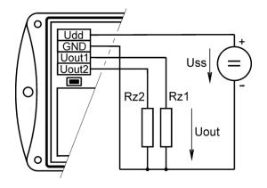
Maximum load current of each voltage output is 0.5 mA
