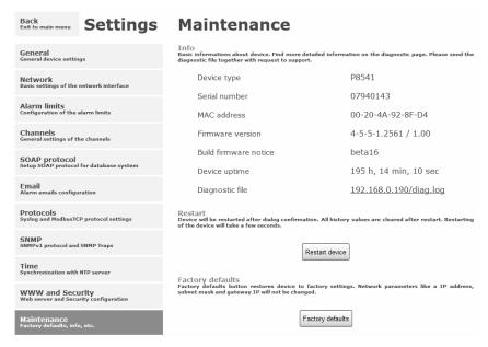
Network parameters are changed while you close jumper inside the device. After jumper closing it is necessary connect power supply. Factory defaults have no effect to user correction inside probe.
